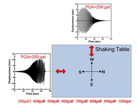
Figure 14. The E-W and N-S components of displacement time histories of the artificial earthquake with the PGA equal to 250 gal.
